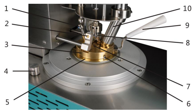
1 Stirrer 2 Igniter 3 Test cup cover 4 Gas control valve 5 Test cup 6 Test cup cover pin 7 Shutter plate 8 Windshield 9 Test cup handle 10 Integrated temperature sensor
