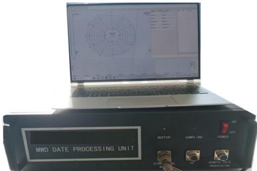
The ground system of oilfield drilling measurement instruments is the core platform for achieving geological guidance and real-time monitoring of drilling parameters, which is divided into two modules: ground data processing instrument and software processing system.
