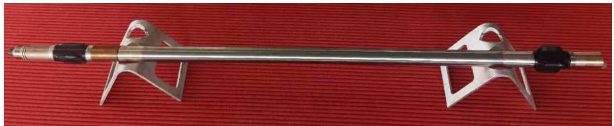
As is well known, one of the main functions of MWD is to measure the geometric parameters of the wellbore. Directional well engineers will adjust the actual drilling trajectory based on real-time uploaded inclinometer data to achieve the expected design trajectory effect.
